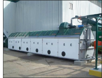
Photo 5-24: Agitated container system © CH2M HILL
