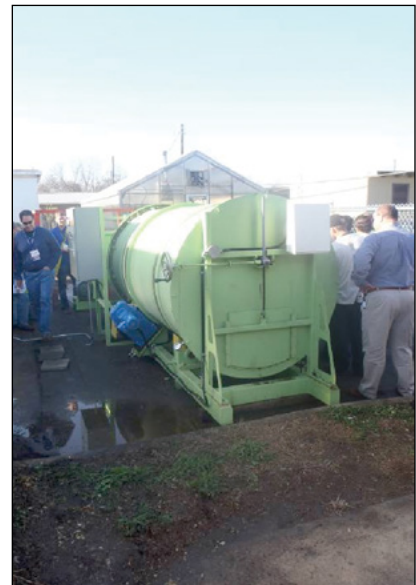
Photo 5-28: Small-scale rotating drum system © CH2M HILL
