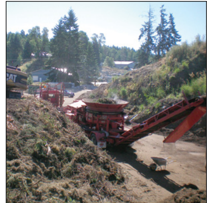
Photo 11-10: Tub grinder © CH2M HILL
