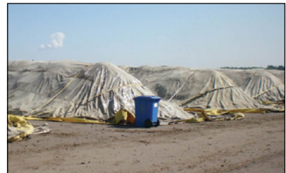
Photo 5-15: Covered, positively aerated composting system © CH2M HILL
