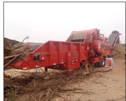
Photo 11-11: Horizontal grinder © CH2M HILL
