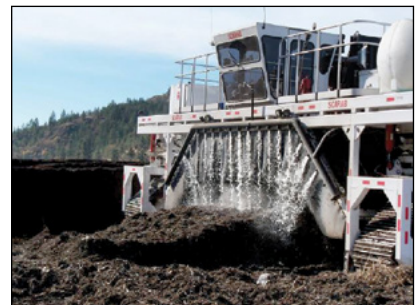
Photo 5-3: Water is best added to windrows when they are being turned © CH2M HILL
