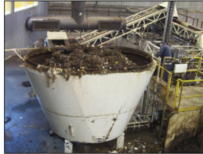
Photo 11-3: Vertical auger mixing unit © Scott Gamble
