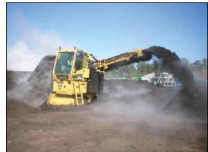
Photo 5-9: A self-propelled windrow turner used for turned mass bed composting © CH2M HILL
