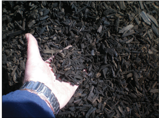
Photo 3-2: Large particles removed from compost through screening can be reused if not contaminated © CH2M HILL
